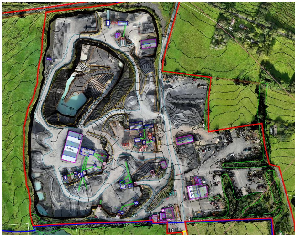
Figure 12: Extract from Drawing No. MM250709-06 of current layout – quarry blasted between October 2015 and December 2019 is clearly visible
